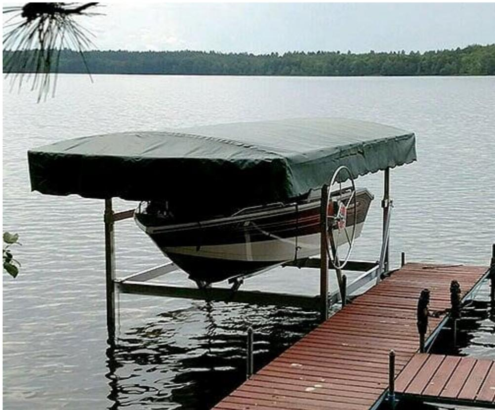
The Craftlander Canopy System consists of the canopy legs, canopy frame, canopy fabric and the canopy fabric attachment system. The canopy fabric attachment system is made up of bungees for the sides and ropes for the ends of the fabric.
